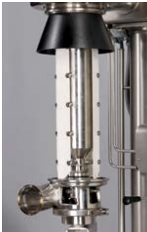
Hydraulic lift and blade funnel for easy maintenance
